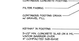
TYPICAL WALL SECTION
